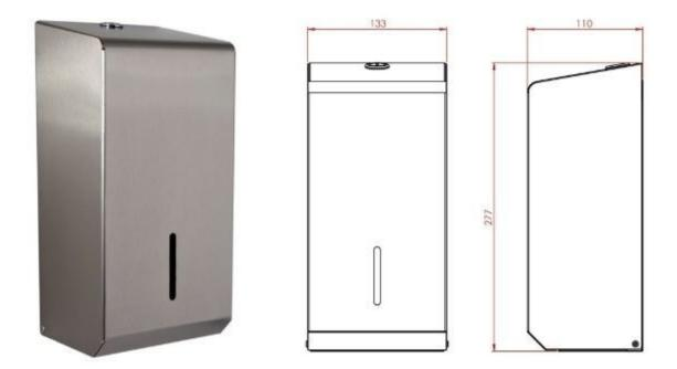
Model WA7014 is our wall mounted multiflat toilet tissue dispenser to hold the capacity of 600 sheets of multiflat tissue paper. Manufactured from grade 304 stainless steel polished to a satin finish. Hinged lockable lid fitted with tumbler lock.
